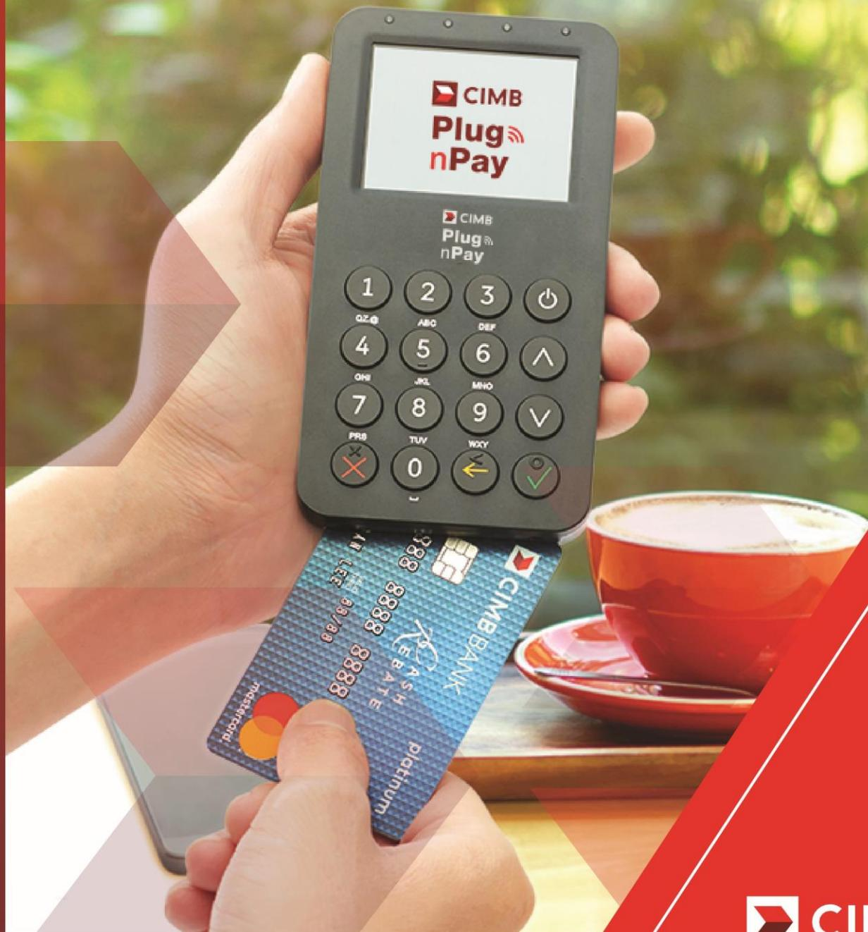
Your CIMB Plug n Pay device is battery operated. It is important to keep the device constantly charged. Charge your device at least once every 14 days. When the device displays a “BATTERY LOW” sign, it does not have enough energy to continue operations, and must be charged immediately.
